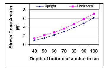
Observations of stress cone failures such as the photograph to the left in snow that has been manually compressed do not show clean shears of the entire cone. Weaknesses obviously exist inside the compacted snow, which mean that the actual shear surface is less than the theoretical area and therefore the strength will also be weaker than the maximum theoretical strength. However failures under shear are still relatively strong when compared to anchors failing under compression.
