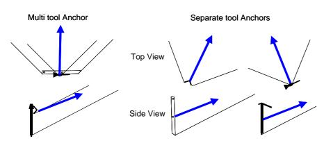
When there is a need to produce a stronger anchor than can be built with a single piece of equipment a multiple point anchor can be built. If the pieces of equipment are put in close to each other then an issue occurs with overlapping stress cones. Although
