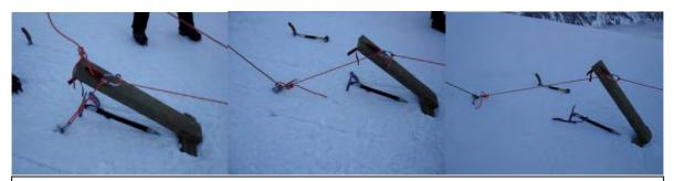
Simulated belayer in the system. From left to right. 0.0 m, 0.5 m, 1.0m back from belay point. All photos were taken at point of failure
