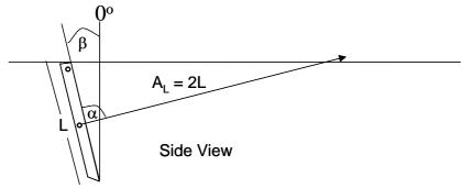
The depth of the bottom of the upright mid clip has a major effect on the size of a stress cone in stronger snow. The size of the stress cone decreases the further a stake is leaned back. This would weaken the anchor in strong snow.
