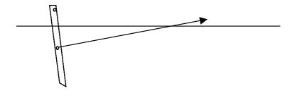
This style of anchor requires a wire cable attachment to the centre of the stake.
