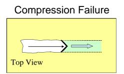
In compression failure the anchor pulls forward through the snow. Under a steady load this can be a fairly slow movement. The compression strength of a snow anchor is dependent on the compression strength of the snow, the size of the buried object and whether the load is evenly spread over the buried object.
